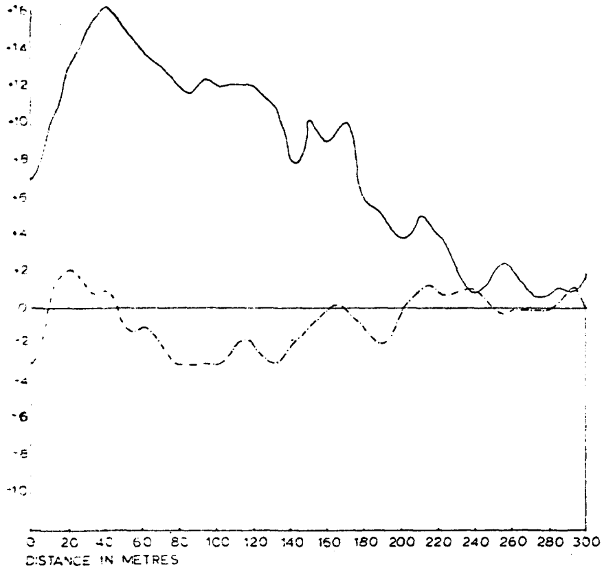
FIG. 18 V.L.F. EM. Traverse 3 Transmitter NAA Station Interval 10M Real Component — Quadrature Component - - - Direction of Readings →
